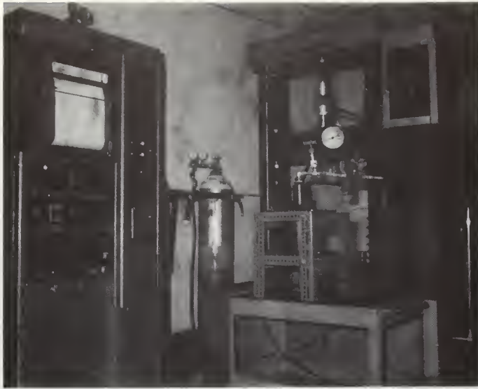
FIGURE 1. BIAXIAL TESTING APPARATUS, SHOWN LEFT TO RIGHT, INSTRON CABINET, NITROGEN CYLINDER WITH REGULATOR VALVE, HYDRAULIC ACCUMULATOR FLASK WITH VALVES AND HYDRAULIC PRESSURE GAUGE, AND INSTRON GRIPS WITH BIAXIAL COMPRESSIVE SPECIMEN BETWEEN THE CROSSHEAD AND LOAD CELL.
